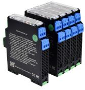
RS485 half-duplex input /RS232 output 1 input 1 output
